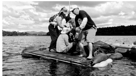
Fig. 2 – Gravity and piston coring in November 2017 on an improvised platform on Biển Hồ maar lake from water depths up to ~21 m.
